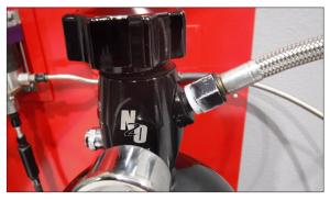
Allow the nitrous to leak until the hose is un pressurized and disconnect the hose.
