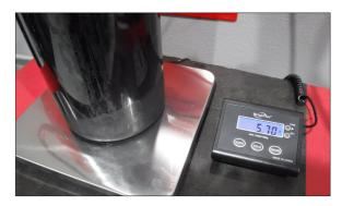
• The nitrous pressure will equalize between the mother bottle and the bottle you are filling. Watch the weight on the scale to make sure it does not over fill the bottle.
