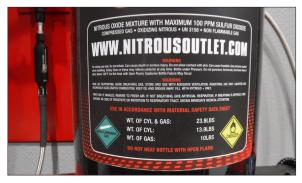
The nitrous bottle you are filling should have a label on the bottle that states the empty weight and a full weight.
