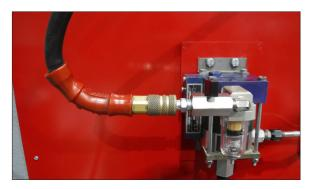
• Connect the air supply to the nitrous pump.
