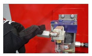
• When the scale reaches the weight needed close the shut off valve to the air supply on the pump.
