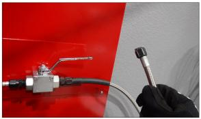
If you are not filling another bottle, Hold the nitrous hose firmly and slowly bleed nitrous pressure from the feed pump by partially opening the inline shut off valve.
