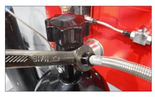
• When the discharge switches from clear air to a solid white nitrous cloud tighten the feed hose.
