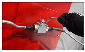
• Partially open the inline shut off valve, slowly.
