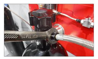
• Loosen the hose at the bottle valve you are filling.
