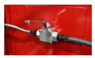
• Close the inline feed hose shut off valve.
