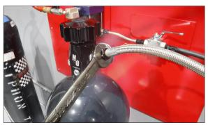
• Using a wrench, slowly loosen the feed hose at the bottle valve you are filling until it starts leaking.
