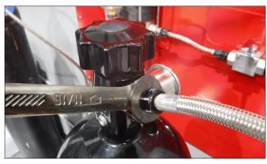
• Using a wrench, tighten the pump station feed hose to the bottle valve on the bottle you are filling.
