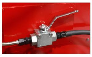
• Slowly open the inline shut off valve until it is fully open.
