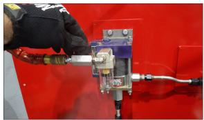
• Once the gravity filling process stops open the air supply shut off valve to activate the pump.
