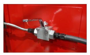
Make sure the pump station's inline shut off valve is closed.
