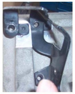
Reinstall stock bracket using stock bolts. You must grind a little material away from the bottom bolt area and just below the 2nd bolt area.
