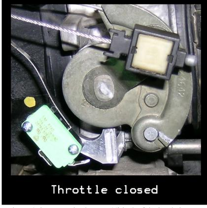
Step 5: Using a pair of quality wire strippers/crimpers, strip about an 1/8 inch of the insulation away from your two activation wires. Install one wire per terminal as shown. After crimping, tug on the wire: it should not come out. If it does come out you did not have a proper crimp. Reinstall and try again. Now install one wire assembly on each
