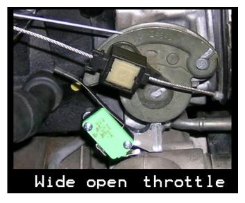
Step 4: After installation is complete, have a friend push the gas pedal to wide-open throttle. The throttle cam should come into contact with the switch arm right before full throttle is achieved. If the throttle cam makes contact with the arm but does not close the switch contacts at wide open throttle, simply tweak or adjust the arm so it does.
