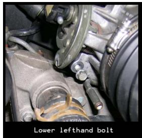
Step 1: Remove the lower passenger side throttle body bolt using your 10mm wrench or socket/ratchet.
