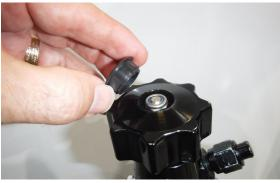
**Step 1:** Remove the plastic cap on top of the bottle valve.
