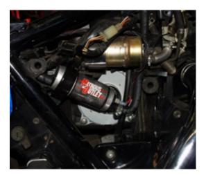
With the "T" fitting installed, use the rubber fuel line and clamps that are included in your system to connect to "T" fitting to the inlet nipple of the enclosed fuel filter, use the rubber hose and clamps to connect the outlet of the fuel filter to the inlet of the fuel pump. Now, use the enclosed rubber hose and clamps to connect the outlet nipple of the fuel pump to the fuel solenoid inlet nipple. Double check all your fuel line connections and clamps.
