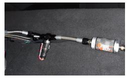
• Install the pressure switch into the female 1/8" NPT port of the manifold. Connect the nitrous feed line to the AN portion of the manifold.
