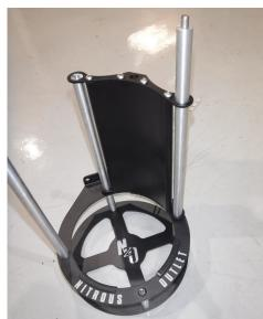
• Slide the large holes of the extrusion bracket over the middle bar and side bar of the Race-Light bracket. The extrusion bracket works on either side of the Race-Light bracket. It is your choice as to which side the electrical wiring needs to be located.
