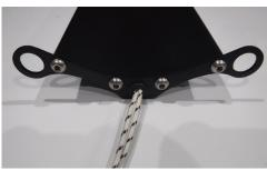
• Using a 5/32" Allen wrench, attach the extrusion bracket to the bottle cradle with 4 stainless steel  $\frac{1}{4}$ -20 x 1/2" long button head cap screws.
