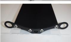
• On the opposite side of the bottle cradle, use a 5/32" Allen wrench, attach the other extrusion bracket to the bottle cradle with the remaining 4 stainless steel 1/4-20 x 1/2" long button head cap screws.
