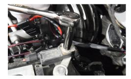
• Connect the black 10ga wire leading out of the relay to the negative battery terminal or a known good ground.
