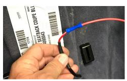
Double check all connections that you completed by giving a slight tug on both ends of the connection after the heat shrink is complete or the pins and connectors have been installed. The goal on installing the harness is to complete this process with a clean and secure attachment of all wiring connections, making sure they are not subject to damage due to heat or moving parts.
