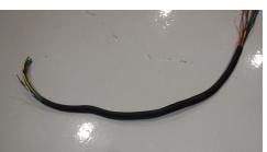
• Feed the section of sleeving from the component end of the harness toward the relay. The best procedure for this is to feed all the sleeving onto the end of the harness. It will look like a compressed spring on the harness.
