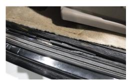
• After you have completed sleeving and heat shrink for each lead, reinstall the harness in its permanent mounting place.
