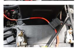
• Install the provided inline 30 amp fuse to the red power source wire. Strip a small setion off the end of the wire, crimp into the provided connector, and heat shrink the connetion. Do not connect to the bettery at this time.
