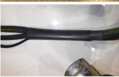
• Secure the taped ends of the sleeving to the harness with heat shrink. The heat shrink should cover the tape and a couple inches on both sides of the tape ring.
