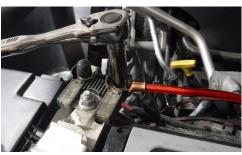
• Connect the red 10ga wire from the 30A fuse connector to the positive battery terminal or positive voltage supply.
