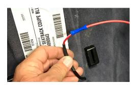
Double check all connections that you completed by giving a slight tug on both ends of the
