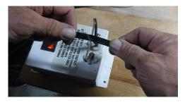
• Cut all sections of sleeving with a hot knife. This will melt the fibers of the sleeving together so that is does not unravel while installing it on the harness.
