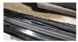
After you have completed sleeving and heat shrink for the harness, reinstall it in its permanent mounting place.
