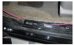
Route the wires to your bottle location and secure them in place. It is recommended to follow your existing harness for easier routing and any possible firewall penetrations.
