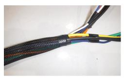
• Using electrical tape, tightly anchor each end using no more than 1 ½ rounds.
