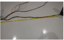
• To cut a specific length of sleeving, begin at the relay and measure up to the branch. Make sure to add 6 to 8 inches to the measured length due to the fact that the sleeving will shorten as it expands over the harness.
