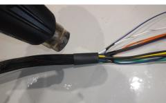
• Secure the taped ends of the sleeving to the harness with heat shrink. The heat shrink should cover the tape and a couple inches on both sides of the tape ring.
