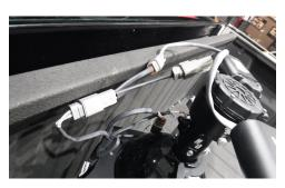
• Connect bottle opener wires from the existing harness to the Y connector.
