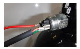
Add the nitrous pressure switch wire from the DIY harness to the connector on the non-powered wire on the pressure switch of your system.
