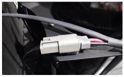
• Connect the heating element for the second bottle.
