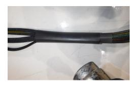
Using heat shrink, cover the breakout or the branch off to ensure you have no exposed wires.
