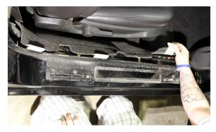
**Step 8:** Unclip the passenger side carpet and roll it back toward the passenger seat.
