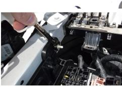
• Using a 10mm wrench, remove the nuts connecting fuse box to the top of the fender.
