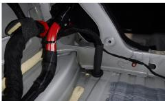
• Route the wiring harness through the drilled hole in the trunk floor. Once the harness is completely through the hole, slide the 1-1/4" grommet into place to protect the harness. The grommet is on the harness.
