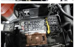
• Using a flathead screwdriver, disconnect the 5 fuse connectors from the fuse box.
