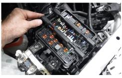
• Use the handles to remove the fuse panel from the fuse box.
