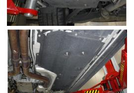
• Reinstall the passenger side under car panel.
