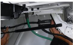
• Continue routing the dedicated tank harness along the upper passenger side of the trunk. Using 2 of the provided 1/4" P-clamps, #10-16 x 1/2" long self-tapping screws, and a 5/16" socket, secure the harness to the passenger side trunk wall. (Rear seat back removed for clarity, not necessary.)
