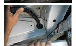
• Install a provided 1-1/2" grommet in the body crossmember hole on the fender well side. Pull the wiring harness through it.
