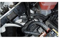
• Using a 10mm socket and extension, remove the nut connecting fuse box to the fender.
