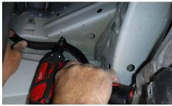
• Route the harness along the rear of the inner fender well and up into the engine bay behind the strut tower. Use a provided 1" P-clamp, #10-16 x 1/2" long self-tapping screw, and a 5/16" socket, to secure the harness to the triangle gusset.
