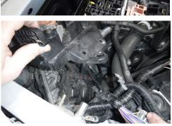
• Under the hood, on the passenger side of the car, in front of the strut tower is the fuse box. Underneath that are the ECM connectors. Unplug the X1, X2, and X3 connectors.
