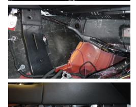
Route the switch panel wiring along passenger side floorboard and to the center console. Tuck
