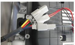
• Route the wires for the solenoids up along the firewall and across the passenger side valve cover to the front of the engine. Use the installation guide in the back of these instructions to put the connectors on your solenoids. After the connectors are installed, plug them in to the leads of the wiring harness. There will be separate leads labeled 'Nitrous', 'Fuel', and 'Purge'.
