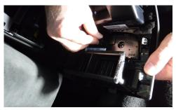
• Reinstall the rear control panel, making sure to reconnect the 2 electrical plugs.
