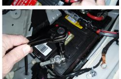
• Reconnect the negative battery cable, include the wiring harness ground wire.
