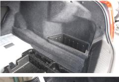
• Reinstall the passenger side trunk panel.
