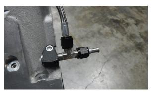
**Step 10:** On the forward facing end of the tee, install the hardline hose barb.
