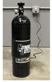
**Option 2.** When choosing Option 2, plug the 110 volt cord into a 110 volt socket plug. **WARNING:** When using the 110 volt plug, monitor bottle pressure closely, heater element can over heat bottle.
