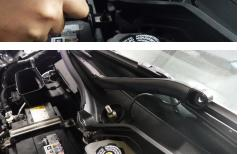
• Using a 14mm socket, remove the nut holding the wiper and lift the wiper up and place it out of the way..
