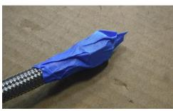
• Cover both ends of the steel braided feed line with tape to prevent debris from getting in.
