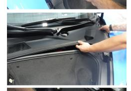
• Remove the main panel covering the battery by pulling it from the clips securing it to the body.
