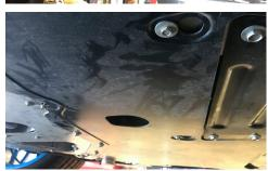
• Under the car, reinstall the rear panel.
