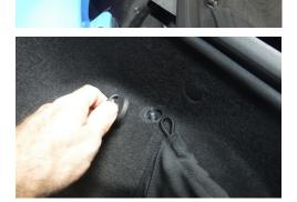
• Unscrew the 2 rear tabs holding the storage net.
