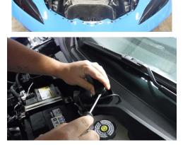
• Using a flathead screwdriver, remove the cap at the base of the passenger side windshield wiper.
