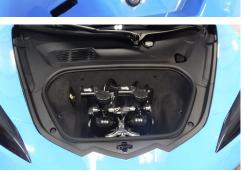
• Reinstall the 4 trim panels around the front storage compartment.
