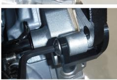
• Using a 6mm Allen wrench, install the M10-1.5 x 16mm bolt through the adapter and into the threaded boss on the water pump.
