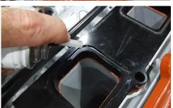
• Using your finger, apply a thin film of black RTV silicone around each cylinder head runner to adhere the provided intake manifold gasket to the cylinder head.
