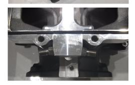
• Place the intake manifold lid on top of the spacer plate. Using a 5mm Allen wrench, install the supplied M6-1.0x45 bolts to fasten the lid and spacer plate to the base.
