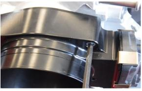
• Using a 5mm Allen wrench, remove the 4 bolts holding the throttle body and remove it from the vehicle.
