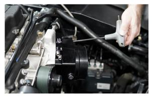
• Using a 5mm Allen wrench, install the nitrous plate between the throttle body and intake manifold with the provided 6mm bolts.
