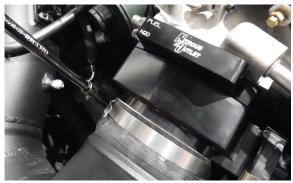
• Reinstall the intake air tube.
