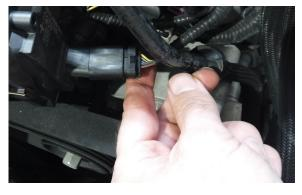
• Disconnect the throttle position sensor.
