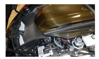
**Step 23:** Reinstall the engine cover.
