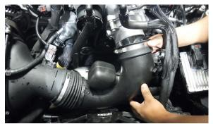
**Step 21:**Reinstall the intake tube and reconnect the PCV line.
