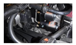
**Step 20**Reconnect the throttle position sensor.
