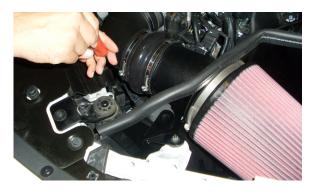
**Step 11:** Reinstall the intake tube.
