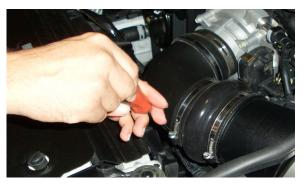
**Step 3:** Using a flathead screwdriver, loosen the hose clamps on the intake tube then remove the tube from the vehicle.
