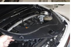
• Using a flathead screwdriver, remove the radiator cover panel by releasing the pins on each side, then pulling it from the retaining clips.
