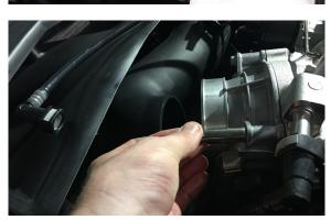
• Using a 10mm socket, remove the 4 bolts holding the throttle body and remove it from the vehicle.
