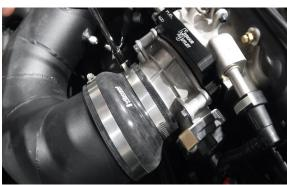
• Reinstall the intake air tube.
