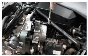
• Using a 10mm deep socket, install the nitrous plate between the throttle body and intake manifold with the provided 6mm bolts.
