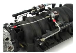
78mm FBody/GTO/Corvette plate fittings face back toward the firewall
