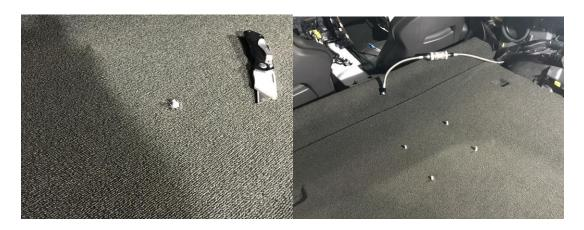
**Step 7:**Once the interior of the car is replaced, you can mount the bottle bracket to the exposed studs.
