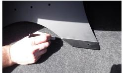
• Mark the carpet for slots that the bottle mount will slide through and slide the carpet out from under the bottle mount.
