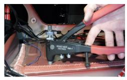
• Using a rivet nut tool, install the 1/4-20 thread Rivet Nuts in the drilled holes. For more detailed instructions on how to install Rivet Nuts, see the instructions on page 4 and 5.
