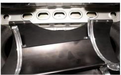
• Reinstall the floor/ spare tire cover then install the bottle mount using the top 4 bolts only.
