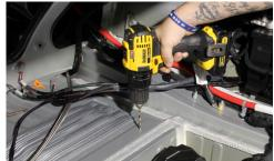
• Check under and behind all areas before drilling to ensure it is free and clear of any component that could be damaged. If it's clear, use a 3/8" drill bit to drill the holes you marked.
