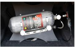
• Lift the spare tire cover to access the mount tabs under the carpet to install the final two bolts in the Rivet Nuts in the floor of the trunk.
