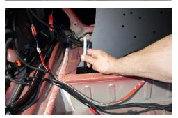
With the floor/spare tire cover out of the vehicle, place the bottle mount in the trunk, centered, with the top of the mount against the rear seat brace, mark the six holes on the bottom of the mount. Next, mark the holes on the top of the mount.
