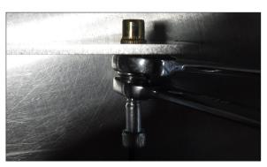
**Step 3:** Use both the 7/16" and ½" wrench. Hold the ½" wrench still and tighten the ¼-20 nut till it stops.
