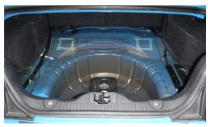
**Step 2:** Remove the floor/spare tire cover.
