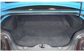
**Step 8:** Reinstall the floor/spare tire cover.
