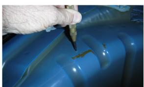
**Step 5:** Using a center punch, mark the 5 hole locations.
