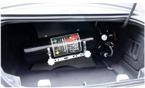
**Sideways Mounting** - When mounting the bottle sideways, the bottle nipple must be angled around 45° downward, toward the rear of the vehicle. This position will orient the siphon tube at the back side of the bottle where the liquid nitrous will be during acceleration.
