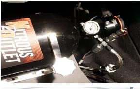
Install the bottle and tighten the feed line onto it with an 11/16" wrench.
