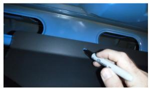
Mark the 3 top and 2 bottom holes with a marker. Remove the bottle mount.
