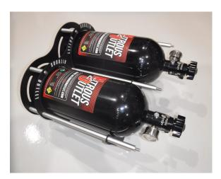
**Step 9:** Place the Nitrous Bottles in the Race-Light bracket.
