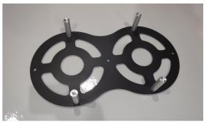
*12lb Carbon bottles* - Have an open circle in the center of the bottom plate. Using the supplied  $5/16-18 \times 1/2$ " button head cap screws, attach the four short support bars to the bottom plate in the four holes on the longest side of the plate, opposite each other.
