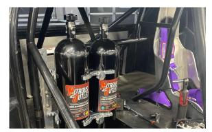
**Vertical Mounting** - If mounting the bottle vertically, the bottle nipple must face toward the back of the vehicle. This position will orient the siphon tube at the back of the bottle where the liquid nitrous will be during acceleration.
