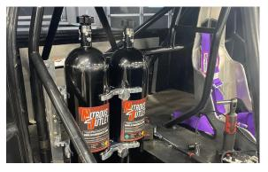
**Vertical Mounting** - When mounting bottles vertically, the bottle nipples must face toward the back of the vehicle. This position will orient the siphon tubes at the back of the bottles where the liquid nitrous will be during acceleration.
