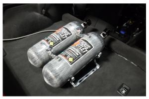
**Lay Down Mounting** - If mounting the bottle in lay down position, the bottle valve must be towards the front of the vehicle with the bottle nipple facing down. This position will orient the siphon tube at the back of the bottle where the liquid nitrous will be during acceleration.
