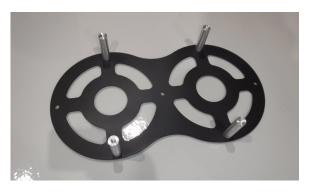
*12lb Carbon bottles* - Have an open circle in the center of the bottom plate. Using the supplied  $5/16-18 \times 1/2$ " button head cap screws, attach the four short support bars to the bottom plate, in the four holes on the longest sides of the plate, opposite each other.
