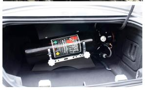
**Sideways Mounting** - If mounting the bottle sideways, the bottle nipple must be angled around 45° downward, toward the rear of the vehicle. This position will orient the siphon tube at the back side of the bottle where the liquid nitrous will be during acceleration.
