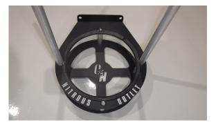
Position the lower support ring so that the mounting tab and Nitrous Outlet Logo are facing to the opposite direction of the bottom plate. Clock the lower support ring so that the two long support bars slide through the larger diameter holes across from one another. Using the supplied button head cap screws attach the front of the lower support ring to the short support bar.
