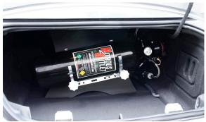
**Sideways Mounting** - If mounting the bottle sideways, the bottle nipple must be angled around 45° downward, toward the rear of the vehicle. This position will orient the siphon tube at the back side of the bottle where the liquid nitrous will be during acceleration.
