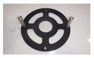
*12lb Carbon bottles* - Have an open circle in the center of the bottom plate. Using the supplied  $5/16-18 \times 1/2$ " button head cap screws, attach the two short support bars to the bottom plate, opposite each other.
