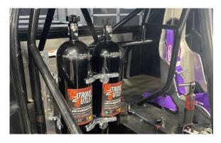
**Vertical Mounting** - If mounting the bottle vertically, the bottle nipple must face toward the back of the vehicle. This position will orient the siphon tube at the back of the bottle where the liquid nitrous will be during acceleration.
