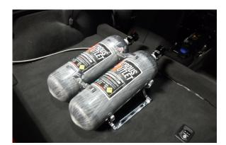
**Lay Down Mounting** - If mounting the bottle in lay down position, the bottle valve must be towards the front of the vehicle with the bottle nipple facing down. This position will orient the siphon tube at the back of the bottle where the liquid nitrous will be during acceleration.
