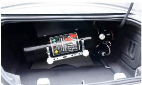
**Sideways Mounting** - If mounting the bottle sideways, the bottle nipple must be angled around 45° downward, toward the rear of the vehicle. This position will orient the siphon tube at the back side of the bottle where the liquid nitrous will be during acceleration.
