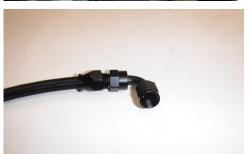
The dedicated tank supply and return hoses will need to have 90° hose ends installed on both ends. For more detailed instructions on how to install hose ends, see the instructions on page 13.
