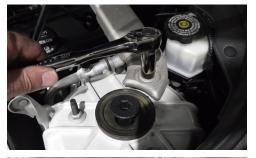
• Using a 13mm deep socket, remove the bolt on the passenger side strut tower crossbrace.
