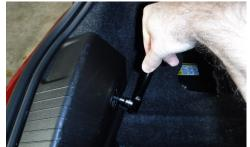
• Using a T-40 Torx bit, remove the screws from the cargo hold-down loops and remove the rear trunk panel.
