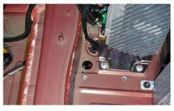
• Using a 1-1/4" hole saw, drill a hole.
