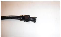
• Put the female side of the hose end onto the fuel hose.
