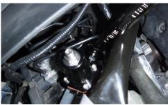
• Connect the return line to the fitting on the bottom of the fuel pressure regulator.
