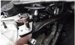
• Using the OEM hardware, mount the fuel regulator on the passenger side strut tower under neath the strut tower brace.
