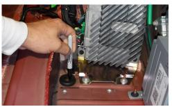
• Center the provided grommet in the flat area forward of the marked line and in between the frame rail and the vehicle electronics. Mark the center of the grommet.
