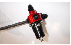
• Using a 5/16" Allen wrench, install the plug in the remaining ports of the fuel pressure regulator. Use blue Loc-tite on the fittings NPT theads.
