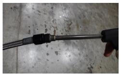
Blow air through one of the dedicated tank hoses and connect it to the fitting on the regulator pointed toward the firewall.
