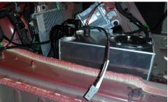
Using the supplied Deutsch connector, connect the wiring for the fuel pump. (See page 12 for connector assembly instructions) Connect the wires for the dedicated fuel system to the dedicated fuel tank.
