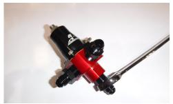
• Using a 3/4" wrench, install the 3 straight 3/8"NPT-6AN fittings as shown on the fuel pressure regulator. Use blue Loc-tite on the fittings NPT theads.
