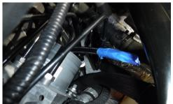
Pull the fuel lines to the Fuel Pressure Regulator in the engine bay and to the fuel tank in the
