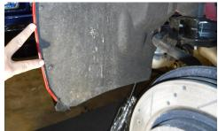
• Jack up the passenger side of the car and place jack stands under the car for safety. Remove the passenger side wheels.
