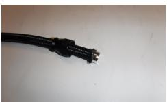
• Put the inner sleeve of the fitting on the end of the hose with the tapered end over the Teflon inner liner.
