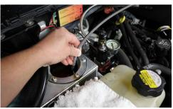
Using a 9/16" wrench, loosen the nut at the top of the fuel pressure regulator. Using a 3/16" Allen wrench, adjust the set screw to achieve the desired fuel pressure. Turn the Allen wrench to the right to increase pressure. Turn the Allen wrench to the left to decrease pressure. Once the pressure is set, use the 9/16" wrench to tighten the nut to lock the set screw in place.
