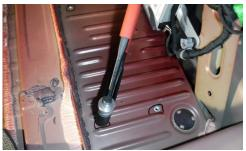
• Using a rivet nut tool, install the 1/4-20 thread Rivet Nuts in the drilled holes. For more detailed instructions on how to install Rivet Nuts, see the instructions on page 14 and 15.
