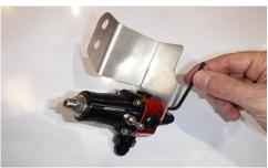
• Using a 9/64" Allen wrench, install the fuel pressure regulator on the provided mounting bracket as shown.
