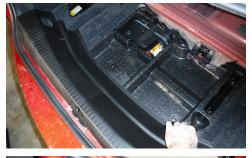
Using a body tool, remove the push pins holding in the passenger side trunk panel and remove
