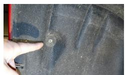
• Using a T-15 Torx bit, remove the passenger side fender liners.
