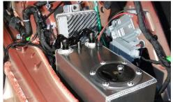
• Connect the supply hose to the fitting to the passenger side of the dedicated tank. Connect the return hose to the driver side of the tank.
