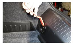
Using a body tool, remove the plastic screw covers located in the center of each cargo D-ring, mounted to the plastic panel at the rear of the trunk.
