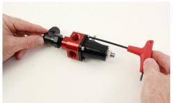
This fuel system is capable of supporting high or low fuel pressure. The fuel regulator currently has the low pressure spring installed. It is designed to supply 3 - 20 psi. If your application requires high fuel pressure you will need to install the supplied high pressure spring. It is designed to supply 20 - 65 psi. To swap the regulator spring, use a 9/64" Allen wrench to remove the 4 cover screws.
