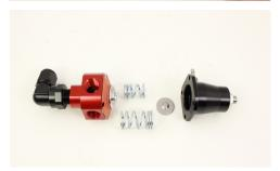
• Remove the top cover exposing the diaphragm, spring and retainer. Swap the spring and re-assemble.
