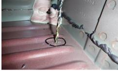
• Check under the area you are drilling to ensure it is clear of any electrical or fuel system components. If it is clear, use a 3/8" drill bit to drill the holes you marked.
