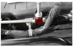
Using the 40" line from a previous step, install one 90° hose end & one straight hose end.
