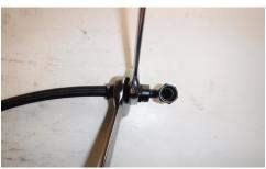
• Using two 3/4" wrenches, thread the male and female ends together.
