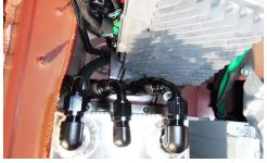
• Using an 11/16" wrench, connect vent hose to the middle fitting on the tank. Run the hose through the 1-1/4" hole with the supplied grommet.
