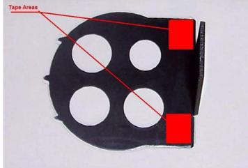
**Step 2:** Place the switch panel onto a piece of paper or poster board. Once you have traced the panel cut it out as shown. This is a template to help locate where you will have to drill the 3 holes
