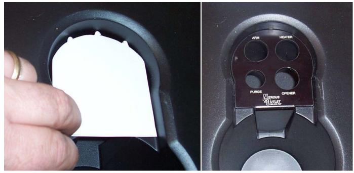
**Step 4:** Route all your wiring for your accessories to the switch panel and make your connections. There is plenty of room under this panel to roll any excess wire under the panel, giving yourself a little extra wire will make your install easier. The long vertical leg is to hide all the wiring from sight.
