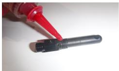
• Apply red Loc-tite on the NPT threads of the nitrous nozzle.
