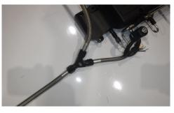
• Using an 11/16" wrench tighten the main feed line on to the Y fitting assembly.
