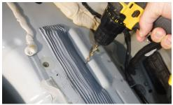
• Check under the vehicle and make sure the area you will be drilling holes in, is clear of any electrical, braking, exhaust, or fuel system components. Then use a center punch to mark the center of your marks. Drill the holes you marked.
