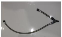
• Using an 11/16" wrench tighten the the 6" & 22" 6AN nitrous feed lines to the provided 6AN Y fitting.
