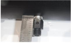
• Make sure the nozzle is firmly tighten in place. In theory there should be 3/16" amount of thread exposed but could vary.
