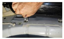
• Place the nitrous bottle back in its desired location. Using a sharple mark the mounting tabs bolt holes. Then remove the bottle from the vehicle.
