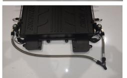
• The 6" feed line should be routed to the side of the vehicle with the main feed line. The 22" feed line should be routed to the other side of the vehicle.
