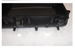
Using a 7/16" wrench, tighten the (6) modified nozzles in the remaining 1/8"NPT ports on the supercharger lid. Make sure to point the discharge hole directly down toward the bottom of the lid. The dimple on the hex flat is aligned with the discharge hole of the nozzle for easier alignment. This will allow the nitrous to inject directly into the intake runners.
