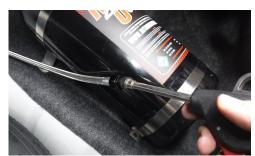
• Remove the tape from both ends of the feed line and blow the hose out with compressed air.
