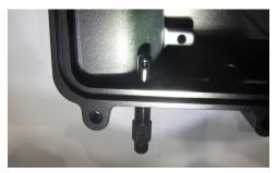
• Using a 7/16" wrench, tighten the (2) <u>unmodified</u> nozzles in the 1/8"NPT ports on each side at the back of the supercharger lid. Make sure to point the discharge hole directly down toward the bottom of the lid. The dimple on the hex flat is aligned with the discharge hole of the nozzle for easier alignment. This will allow the nitrous to inject directly into the intake runners.
