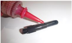
• Apply red Loc-tite on the NPT threads of the unmodified nitrous nozzles.
