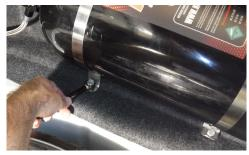
• Place Bottle back in location, make sure the bolt holes line up, and bolt the brackets in place.
