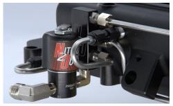
• The hardline for the front nozzle will go above the MAP sensor boss and the harldine for the second from the front nozzle will go under the MAP sensor boss.
