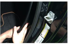
Use a Phillips head screwdriver to remove the single screw under the kick panel. Then use your hands to pull loose the trim next to the backseat on the drivers side. This will be where the nitrous feed hose passes through to the trunk.
