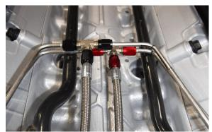
• On the back of the engine, install the 25.5" 3AN - 4AN straight fuel hose to the fuel hardline 3AN tee using a 1/2" wrench. Then install the 22" 3AN - 4AN straight nitrous hose to the nitrous hardline 3AN tee. Route these hoses to the driver side of the engine.
