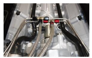
• On the front of the engine, install the 19.5" 3AN - 4AN straight fuel hose to the fuel hardline 3AN tee using a 1/2" wrench. Then install the 20.5" 3AN - 4AN straight nitrous hose to the nitrous hardline 3AN tee. Route these hoses to the passenger side of the engine.
