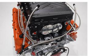
Using an 11/16" Wrench tighten the main feed line on to the Y fitting assembly. The 13" feed line should be routed to the driver's side of the vehicle. The 27" feed line should be routed to the passenger side of the vehicle.
