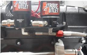
• On the passenger side solenoids, use a 9/16" wrench to connect the nitrous and fuel hoses to the solenoids. The hose with the black b-nut connects to the nitrous solenoid and the hose with the red b-nut connects to the fuel solenoid.
