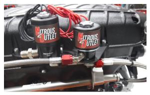
• Using a 9/16" wrench, install the 18" 4AN straight fuel line to the passenger side fuel solenoid.
