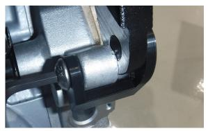
• Using a 6mm Allen wrench, install the M10-1.5 x 16mm bolt through the adapter and into the threaded boss on the water pump.
