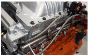
• Using an 11/16" Wrench tighten the 27" feed line on to the passenger side nitrous solenoid.
