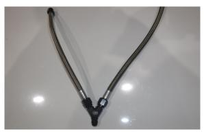
• Using an 11/16" Wrench tighten the the 13" & 27" 6AN nitrous feed lines to the provided 6AN Y fitting.
