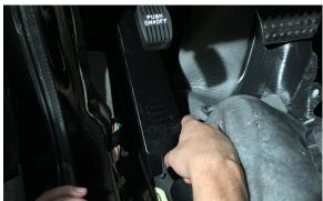
• Use an 11mm socket and wrench to remove the dead pedal under the emergency brake. Once it's loose, remove it from the vehicle.
