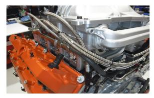
Using an 11/16" Wrench tighten the 13" feed line on to the driver side nitrous solenoid.
