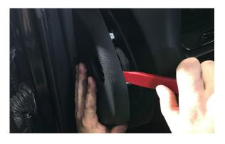
Remove the end cap on the drivers side of the dash using a trim tool. Work the trim tool all around the edges to release all of the clips.
