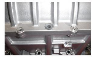
Stack 2 provided washers in the recess for the supercharger mounting bolt. Place one each of the provided 1/2" x 1/8" thick spacers in the recesses for the supercharger lid.
