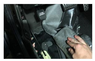
• Locate an open place on the firewall to drill a 1-1/8" hole for the nitrous feed hose to go through. Be sure and check both sides of the firewall to ensure the area you're drilling is clear of anything that can be damaged.
