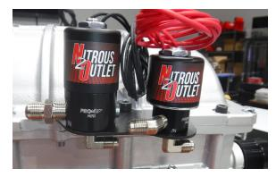
The passenger side solenoid bracket assembly has the inlet and outlet fittings pointed in opposite directions. Reinstall the supercharger mounting bolt through the solenoid bracket. Using a 10mm socket, install the provided M6-1.0 x 30mm bolts through the solenoid bracket and in the supercharger lid.
