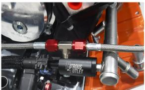
• Using a 1/2" wrench, install the 18" 4AN straight fuel line to the passenger side of the fuel adapter fitting. Install the 27" 4AN straight fuel line to the driver side of the fuel adapter fitting.
