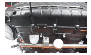
• On the driver side of the supercharger, remove the front three fasteners of the lid.
