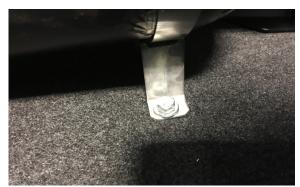
• Mount the bracket, and tighten the bolts with a 5/16" wrench. You may have to have someone under the car with another 5/16" wrench hold the nut while you tighten the bolt. Be sure and use washers on both the bolt and the nut.
