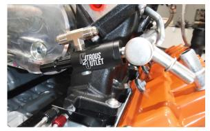
• Install the fuel adapter to the fuel supply line to the passenger side fuel rail by sliding the female end over the fuel line until it to rest against the fuel line flange. Then slide the fuel adapter nut over the fuel line and thread into the body of the fuel adapter. Using a 13/16" wrench tighten the adapter nut firmly into the adapter body pinching the fuel line flange between.
