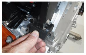
• Insert the support dowel of the Whipple Snout Adapter into the front of the snout support of the Whipple supercharger.
