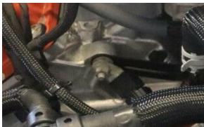
• Using a 10mm wrench, remove the M6 nut on the grounding stud at the back of the driver side cylinder head. Remove the grounding cable and coolant line support bracket from the stud.
