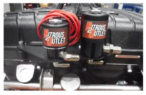
• The driver side solenoid bracket assembly has the inlet and outlet fittings pointed in the same direction. Reinstall the supercharger lid fasteners through the solenoid bracket.
