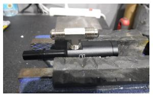
• Apply blue loc-tite on the NPT threads of the 1/8 x 4AN x 4AN branch tee fitting. Then using a 7/16" wrench, install the fitting into the other fuel adapter opening.
