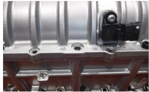
• On the driver side of the supercharger, remove the third from the front mounting bolt and the lid fasteners on either side of the mounting bolt.
