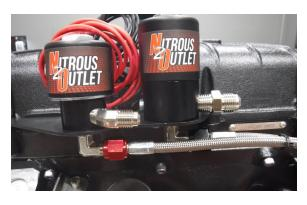
• On the driver side solenoids, use a 9/16" wrench to connect the nitrous and fuel hoses to the solenoids. The hose with the black b-nut connects to the nitrous solenoid and the hose with the red b-nut connects to the fuel solenoid.
