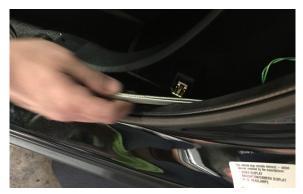
Push the nitrous feed hose behind the trim panel, and into the trunk.
