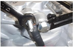
• Install the "L" bracket and grounding cable on the stud on the back of the cylinder head.
