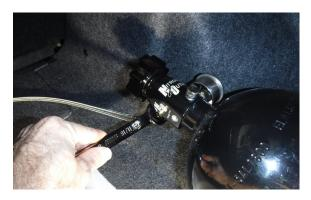
• Tighten the nitrous feed hose onto the bottle with an 11/16" wrench. Do not over-tighten!
