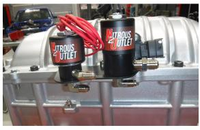
The driver side solenoid bracket assembly has the inlet and outlet fittings pointed in the same direction. Reinstall the supercharger mounting bolt through the solenoid bracket. Using a 10mm socket, install the provided M6-1.0 x 30mm bolts through the solenoid bracket and in the supercharger lid.
