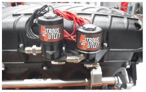
The passenger side solenoid bracket assembly has the inlet and outlet fittings pointed in opposite directions. Reinstall the supercharger lid fasteners through the solenoid bracket.
