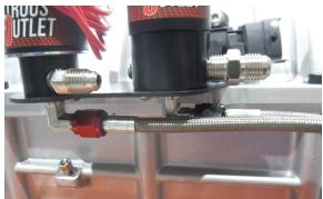
• On the driver side solenoids, use a 9/16" wrench to connect the nitrous and fuel hoses to the solenoids. The hose with the black b-nut connects to the nitrous solenoid and the hose with the red b-nut connects to the fuel solenoid.
