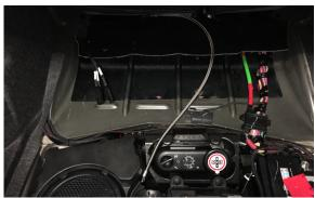
Check the feed hose to ensure it won't be pinched or damaged by the back seat. If there's a chance it could be, relocate the hose to a different spot by routing it under the back seat.
