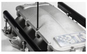
Step 7: Remove the second lid bolt from the front on both sides.
