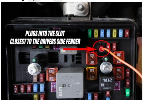
3. Once the fuse is removed you will see two slots, plug the RED WIRE from the unlock cable into the slot closest to the driver's side fender. (Refer to picture below)
