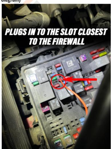
3. Once the fuse is removed you should see 3 slots, plug the RED WIRE from the unlock cable into the slot closest to the fire wall. (Refer to picture below)
