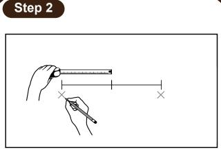
Mark the centre of the wall where you want to place the shelf or mantel and transfer the measurements onto the wall.
