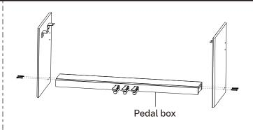
②Use 4 pcs M6x50mm screws to fix the pedal box with left and right stand plate.
