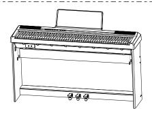
Fixed digital piano on the piano stand with 4 pcs M5X30mm screws.
