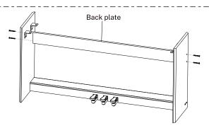
③Use 4 pcs M5x50mm screws to fix back plate with left and right stand plate. Then, the piano stand is completed.
