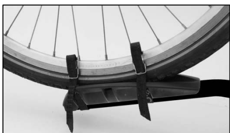
Figure 16: Tensioning straps for front wheel
