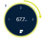
Rotate the controller clockwise until the display is showing the height of the desk. Reset complete.
