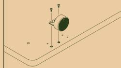
Install the Health Coach Controller (a) to the inserts in the worktop with the Phillips Head Machine Screws (d) provided, as illustrated in the diagram. The Handset can be attached on either the left or right end of the worktop.
