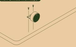
Install the Health Coach Controller (a) to the worktop with the Wood Screws (c) provided, as illustrated in the diagram. The Handset is reccomended to be attached on either the left or right end of the worktop.
