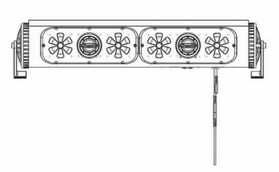
**Step 3.** Plug the BPB-G3's main power cable back in. You will see the flashing LED on the remote go off. Now your remote is paired to the BPB-G3.
