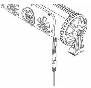
**Step 1**. Remove the power from the BPB-G3 by unplugging the main power cable. Wait 30 seconds
