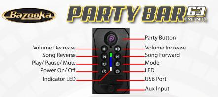
**Mode Button:** Click-press the mode button to toggle between Bluetooth/Aux/USB listening modes. Press-hold to turn off.
