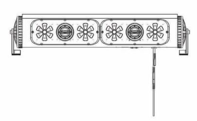
**Step 3.** Plug the BPB-G2's main power cable back in. You will see the flashing LED on the remote go off. Now your remote is paired to the BPB-G2.
