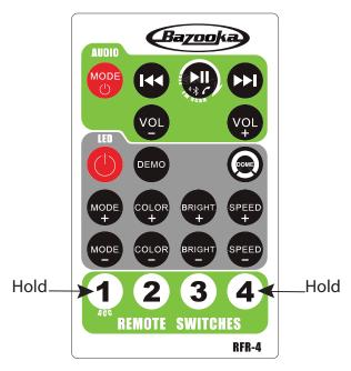
**Step 2.** Press and hold the **1** and **4** buttons. After 5 seconds you will see that the red led on the remote will start to flash slowly. Once the led is flashing release the buttons.
