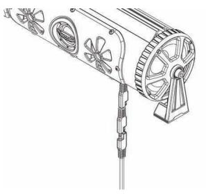
**Step 1**. Remove the power from the BPB-G2 by unplugging the main power cable. Wait 30 seconds
