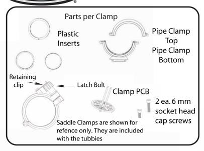
Place clamp on mounting pipe. Minimum distance from edge of clamp to nearest obstruction is 7"(177.8 mm). If clamp is mounted any closer, the Tubbie will not be able to rotate 360 degrees. Make sure clamp is level, then mark pipe so a hole can be drilled for the wires. Hole should be between 1/2" (12.7mm) & 3/4" (19.5 mm). Remove clamp & drill hole.
