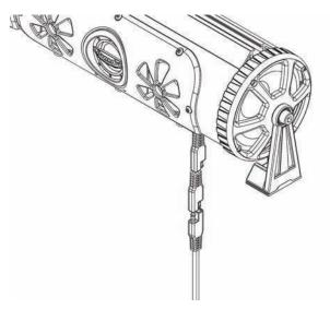
**Step 1**. Remove the power from the BPB24 by unplugging the main power cable. Wait 30 seconds
