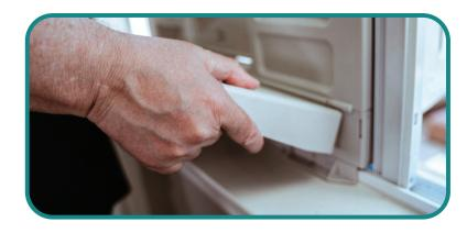
Postition porch tabs at an angle. Then insert porch tabs into back panel slots. Then rotate porch downward and snap porch tabs into bottom panel slots.
