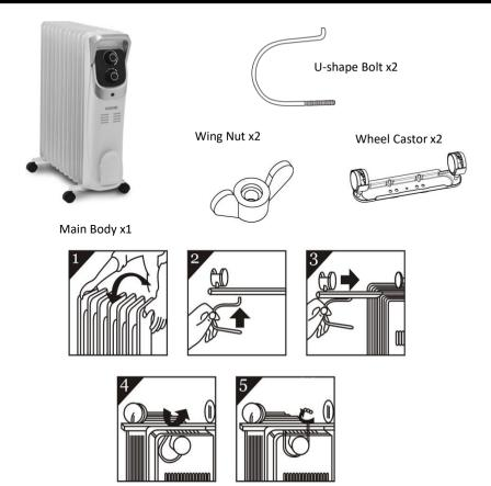
**IMPORTANT:** Please fit the wheel assemblies as per the diagram. Any other position may affect the stability of the heater.
