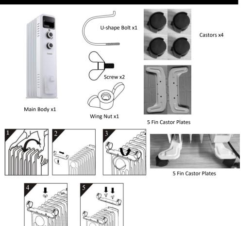
**IMPORTANT:** Please fit the wheel assemblies as per the diagram. Any other position may affect the stability of the heater.
