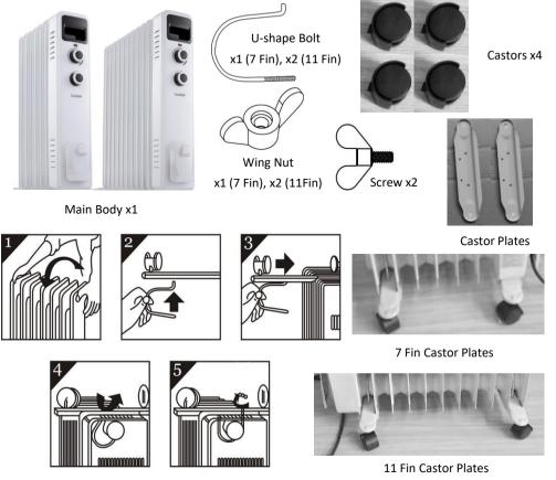
**IMPORTANT:** Please fit the wheel assemblies as per the diagram. Any other position may affect the stability of the heater.
