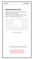
Change 'EZ Mode' to 'AP Mode' by clicking in the top right hand corner Ensure your device's Wifi LED is flashing slowly. If it is not, hold down the "POWER" button for 5 seconds or until the Wifi icon begins to flash. Click 'Confirm indicator slowly blink' and 'Next'
